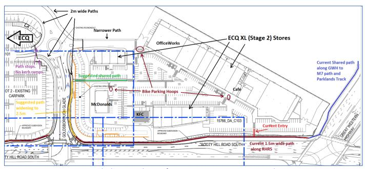
Figure 2 - Marked-up partial copy of Drawing 15766\_DA\_C100, Appendix I page 2.
