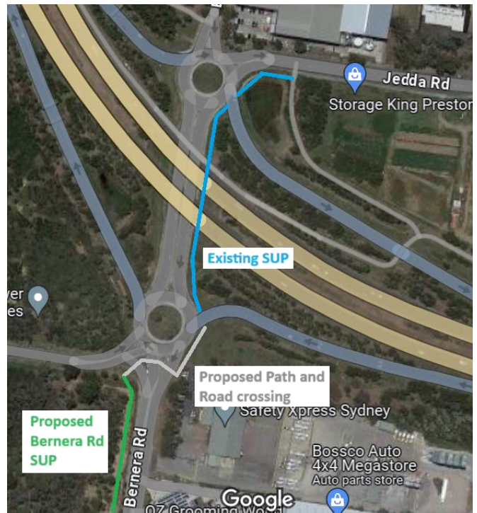
Marked-up Google Satellite View image [3] of the apparent intended AT route across the M7 interchange.
